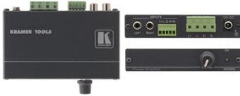
The 900N is a high-performance power amplifier for balanced or unbalanced stereo audio signals. Either input can deliver a speaker output of 10 watts RMS power per channel into a 4Ω load
